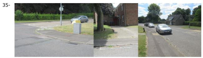
Poor paving by entrance of Denison Rise, the drop-kerb crossing is often impeded here by parked cars. Blocked drain by 24 Barrington Road. Lower end of Barrington Road another drop-kerb crossing, this time to the bus-stop, here blocked. Again, can some scheme to enforce these points be worked up?
